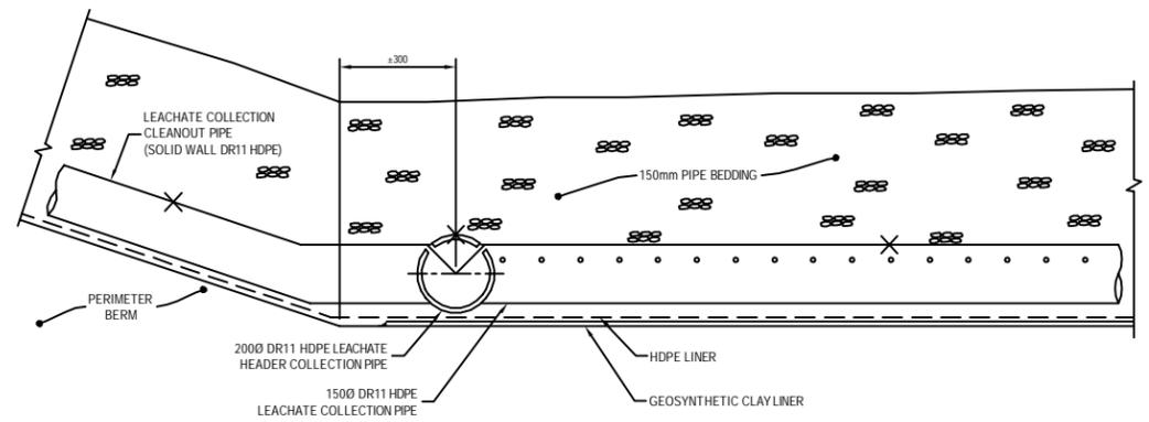
**LEACHATE COLLECTION PIPE AT TOE OF PERIMETER BERM 25**
