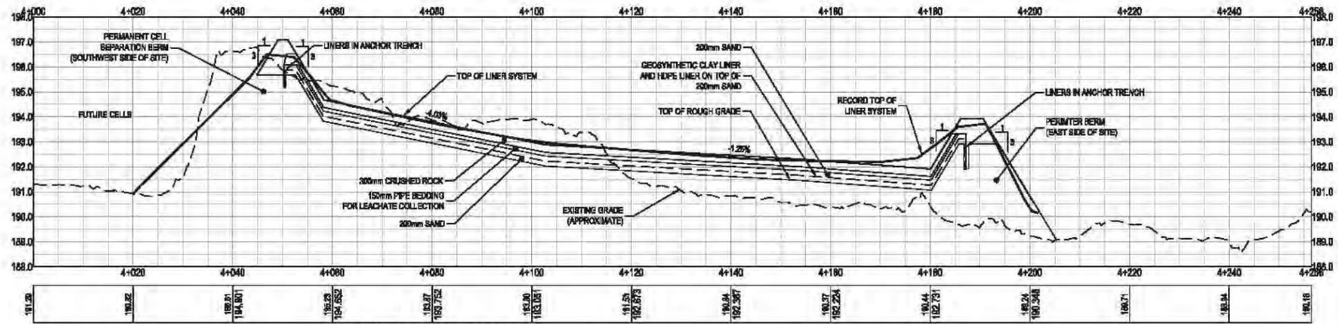
NOTE: ELEVATIONS IN BAND ARE EXISTING ON LEFT AND RECORD TOP OF LINER SYSTEM ON RIGHT
