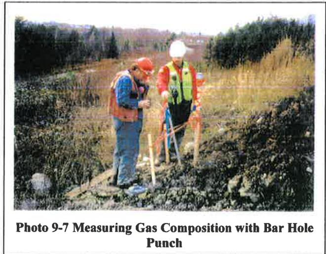
Photo 9-7 Measuring Gas Composition with Bar Hole Punch
