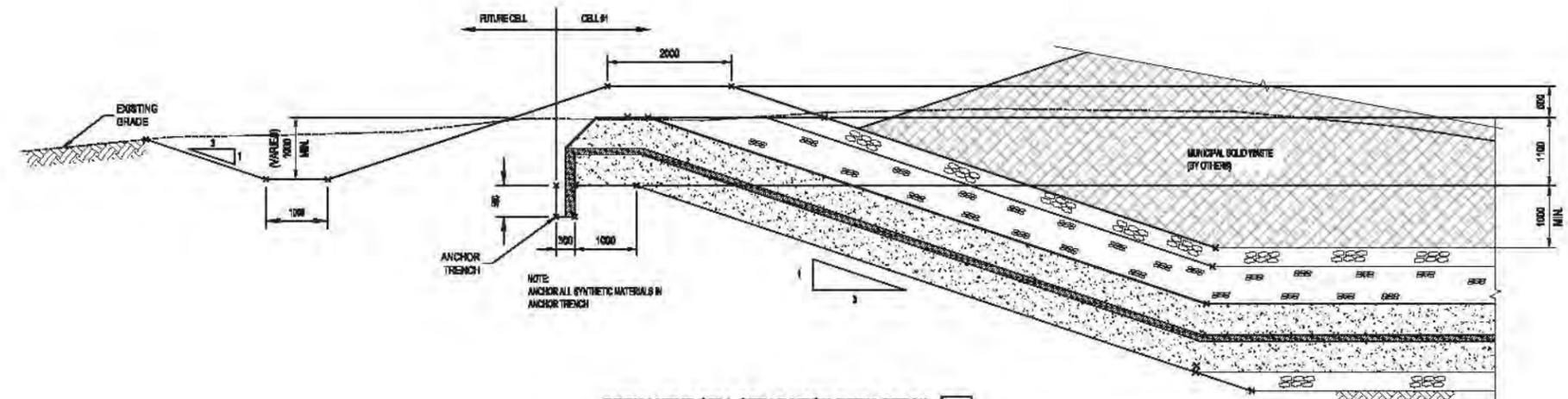
**PERMANENT CELL SEPARATION BERM DETAIL 12**
