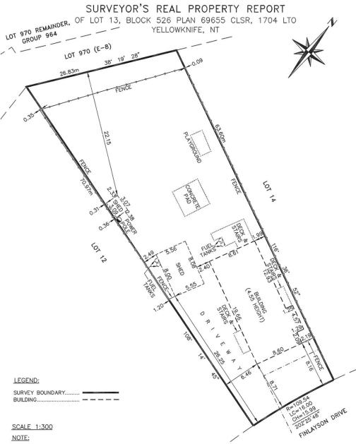
This is not a boundary survey. The boundary dimensions have been copied from PLAN <u>1704</u> LTO. Unless otherwise specified, the dimensions shown relate to the distance from the property boundaries, as described by PLAN <u>1704</u> LTO, to the structure foundation wall at the date of survey.
