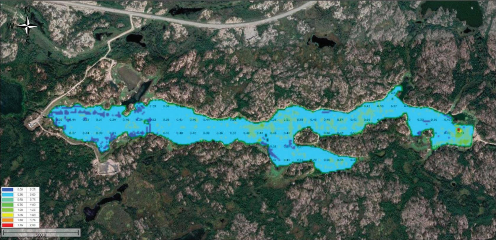
Figure 2 Fiddlers Lagoon sludge thicknesses (m)
